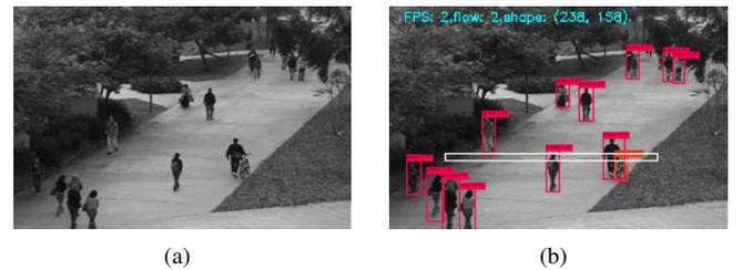
**Fig. 3.** Sample frame of UCSD Pedestrian Dataset. a) original frame of UCSD Pedestrian Dataset. b) output of proposed algorithm, where the white box represents the detection area, the red box represents detected pedestrian.
