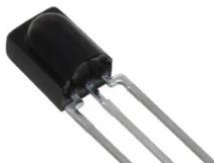
Figure4. The photodetector (TSSP58038) used in the experiment
