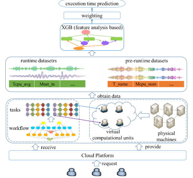
Fig. 1 The procedure of our task execution time prediction model
