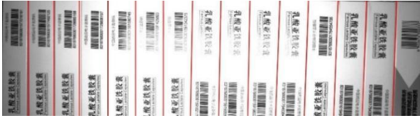
Fig. 4 After filtering, the vertical lines were extracted.
