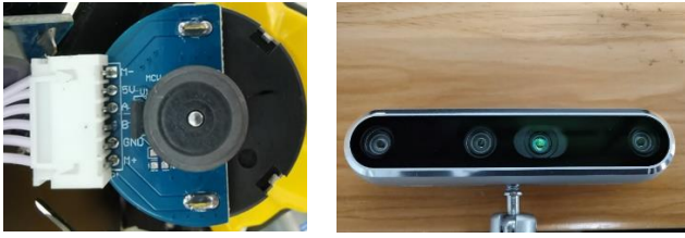
(a) Hall encoder (b) RealSense d455 camera Fig. 4 Physical diagram of mobile robot sensor module
