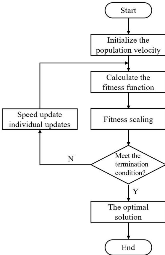
Fig. 2. Procedure of the PSO optimization of SVR parameter.
