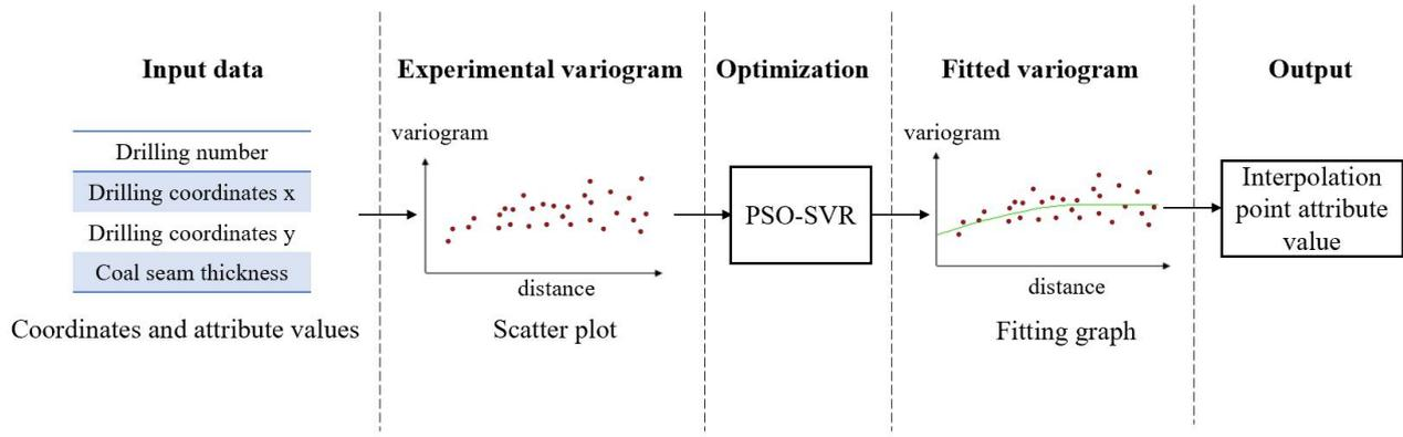
Fig. 1. PSO-SVR optimized Kriging algorithm: an overall structure.
